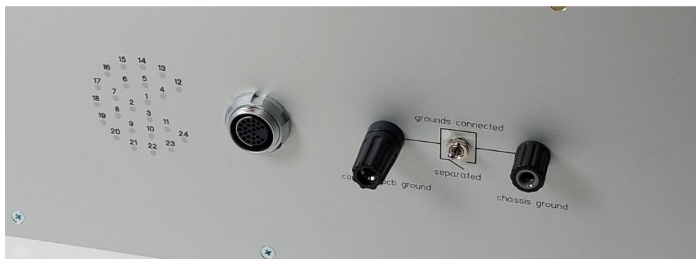
Figure 2: Rear panel switch for grounds connection.
